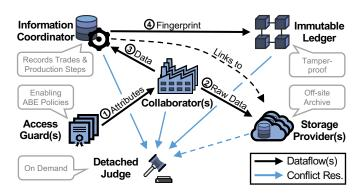
Fig. 1. Our architecture operates as follows. Collaborators retrieve attributes from Access Guards that maintain suitable ABE policies. A dedicated storage provider retains all raw data while a bundle containing a link to the raw data is sent to the information coordinator to securely record all produce and trade operations. A fingerprint of this record is stored on the immutable ledger. In case of inconsistencies, a detached judge can resolve conflicts.
