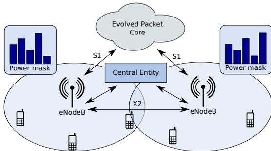
Fig. 1: Schematic overview of the proposed semi-static ICIC.
